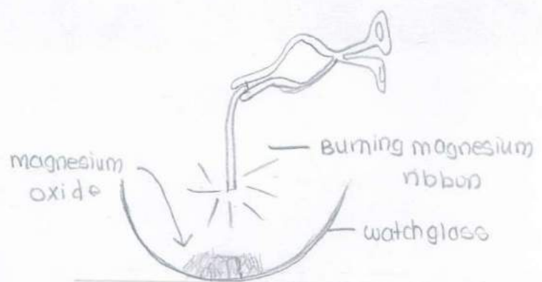
b) magnesium ribbon burns in air to form magnesium oxide.
